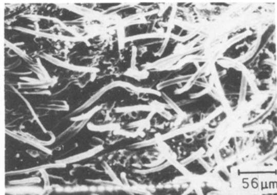
Figure 8 Scanning electron micrograph of the tensile fracture surface of Mix D.
